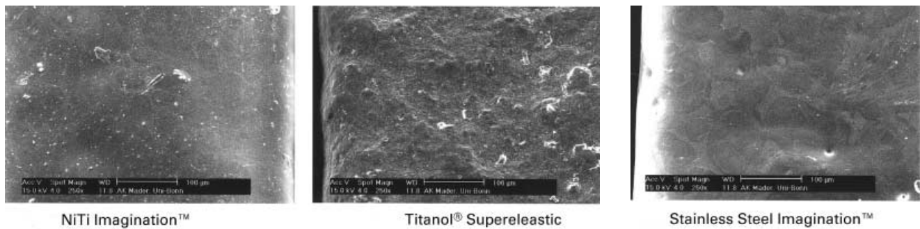
Figure 9b. Surface scans of Teflon® coated wires GNTI, FTSZ, and GSSI.
